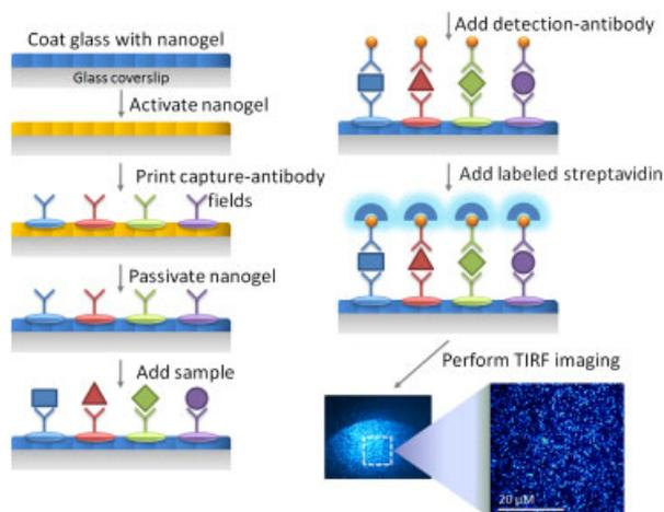
**Figure 1.** Schematic of the single-molecule antibody microarray method.
